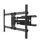
Neomounts WL40S-950BL18 Full motion heavy duty wall mount - 55-110" screen - max 125 kg - VESA 300x200-800x600 - d 8,2-70,3 cm - level adjustment - incl. fixing template - black
