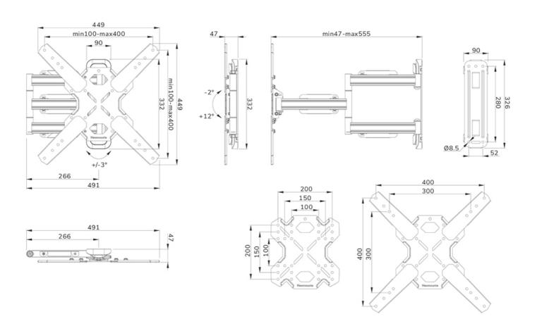
Neomounts Measuring unit: mm
