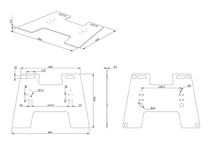
Neomounts Measuring unit: mm
